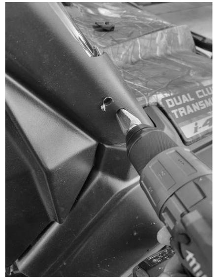
**Step 8.** It may be necessary to slightly enlarge the holes using a step drill bit in the lower OSP cover for proper fit.
