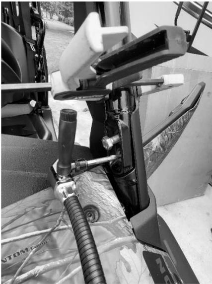
**Step 6.** Loosely install one of the OEM A-pillar bolts into the hole not being drilled to help keep the A-pillar aligned.
