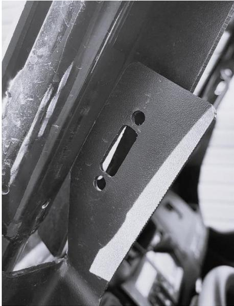
**Step 1.** If installing the A-pod on a vehicle with Honda soft doors previously installed, separate the upper and lower OSP Cover and remove the lower OSP cover.
