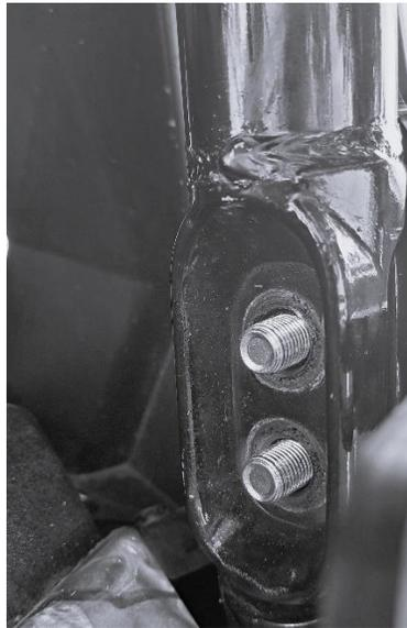
**Step 10.** Install the bolts through the A-Pillar and Loosely re-install the OEM nyloc nuts securing the A-pillar bolts, ensuring they are not cross-threaded. Note: make sure that the mirror is installed before tightening the nuts.
