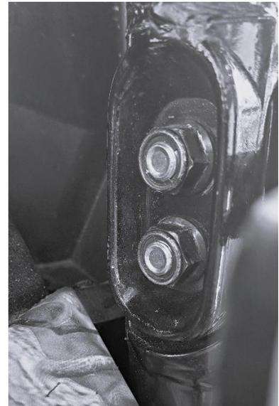
**Step 11.** With the mirror installed, tighten all bolts, and nuts to their specified torque values. Refer to the Service Manual for the torque values of the removed parts. Repeat steps 1-11 on the opposite side.
