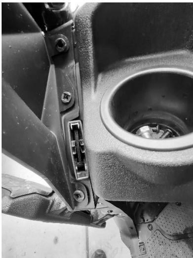
**Step 3.** Reinstall the lower OSP Cover and reinstall the trim clips through the lower OPS cover into the body panels.
