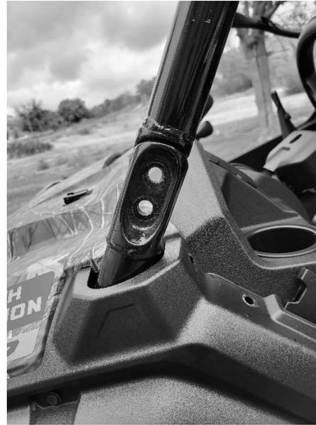
**Step 2.** Remove the vehicle windshield and remove the two OEM A-Pillar bolts and nyloc nuts **on one side of the vehicle.** **Note: You will be reinstalling the nyloc nuts, you will not be re-installing the bolts.**
