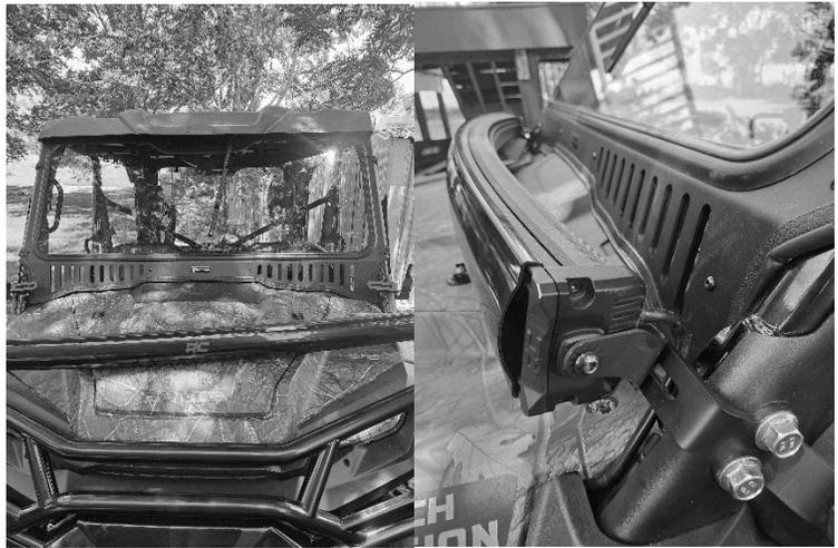
Check installation with the soft door installed and adjust as necessary. Adjust mirror position and torque bolts. Enjoy the use of your new A-Pod mirror and light bar brackets.
