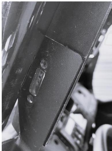
**Step 4.** Check alignment of the lower and upper OSP Covers.
