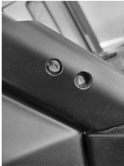
**Step 7.** Drill the holes through the A-pillar and the lower OPS cover with a 12mm or ½ drill bit. If a smaller drill bit is used, make sure the hole through the OSP cover is centered with the A-Pillar hole.
