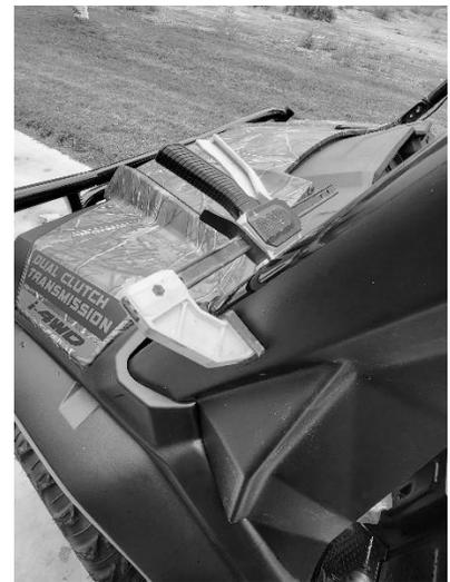
**Step 5.** With proper alignment checked, clamp the Lower OSP Cover to the roll bar.
