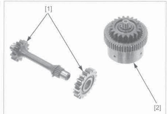
Replace the torque limiter as an assembly.
