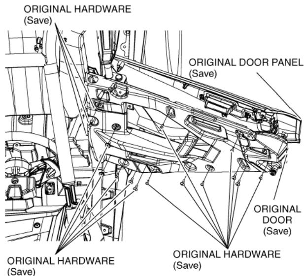
3. Loosely install the driver side Aluminum Door using a 5 x 16 mm button head bolt, washer and spring lock washer.
