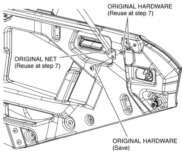
2. Remove original door and hardware. Save for reuse.
