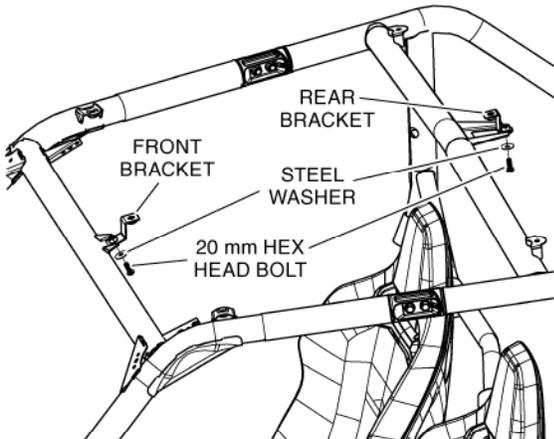
4. Place the aluminum roof over the top of the OPS. Loosely secure the roof in the two center locations using two 20 mm hex head bolts and steel washers as shown. Do not fully tighten the hardware at this time.
