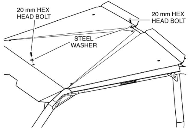
5. Secure the roof in the four outside locations using the original bolts and washers removed in Step 1, as well as two rubber washers in each location. Be sure to tighten all hardware securely.
