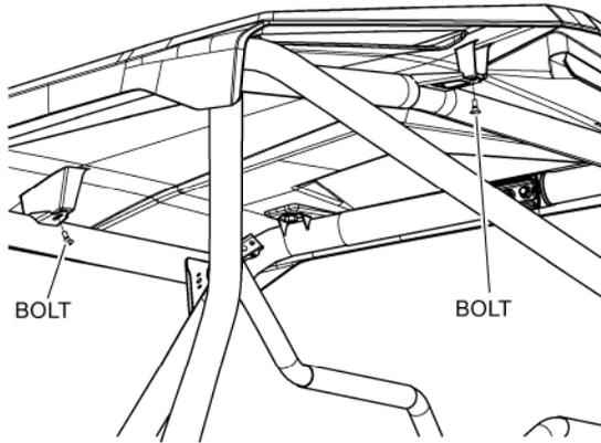
3. Install the front and rear mounting brackets to the inside of the OPS in the locations shown using two 20 mm hex head bolts and steel washers.
