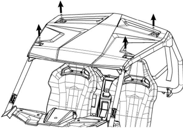
2. Remove the two bolts securing the roof on the inside of the vehicle. Remove the roof and set aside.
