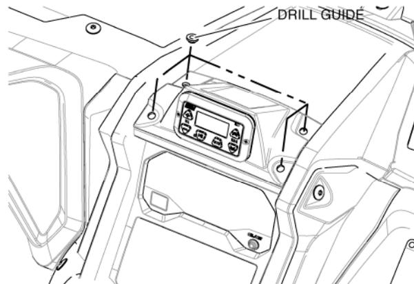
15. Use the drill guides to drill a 1/8 in pilot hole into the instrument panel at the four locations shown.
