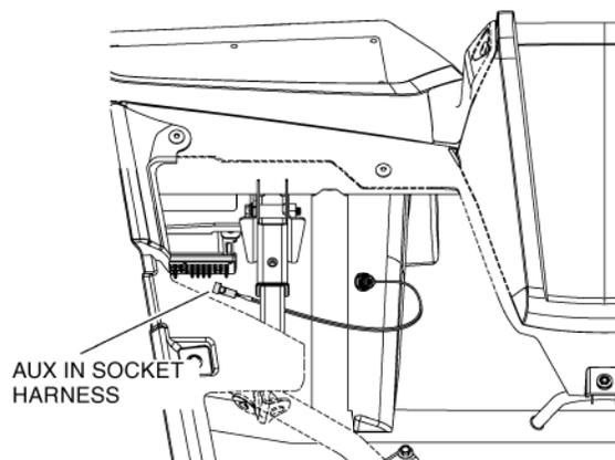
32. Connect the antenna cable to the radio mcu. For best reception, route the antenna cable so it loops back on itself then secure the cable with wire ties (as shown).
