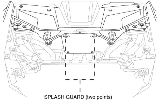
6. Fold down the top portion of the rubber splash guard then remove the dash trim panel.
