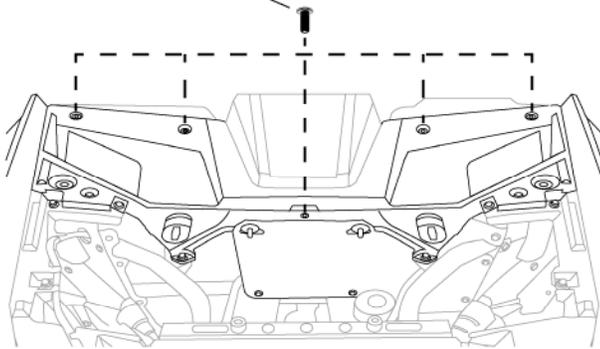
3. Remove the four 10 mm flange bolts (as shown).
