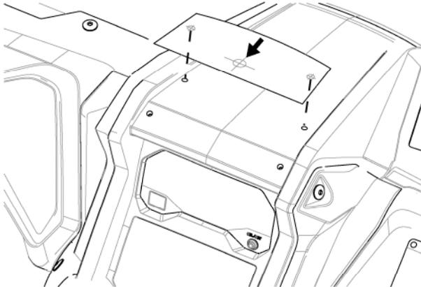
17. Using the 9/16 in drill bit with added tape depth guide prepared previously, drill a hole at the center of your mark.
