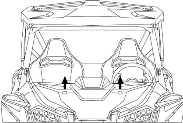
2. Remove the dash trim panel by first removing the five hex head screws (as shown).
