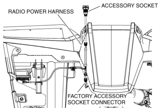
31. Connect the aux in socket harness (previously installed into the glovebox) to the 3-pin connector on the radio mcu. Route the harness under the grab handle mount.
