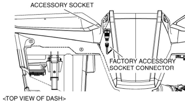
30. Connect the radio power harness to the accessory socket.
