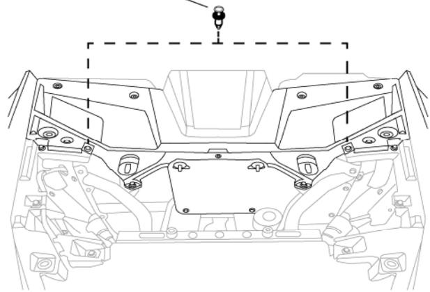
5. Detach the top portion of the rubber splash guard by unhooking it from the two points as shown below.
