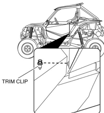
22. Remove the passenger side lower side cover by repeating steps 19 - 20. Remove one 5 mm hex head screw from the rear panel (as shown).
