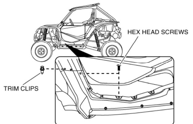
21. Open the driver side door, then use a trim clip removal tool to extract one trim clip located between the door and rear panel of the vehicle. Remove the driver side lower side cover.
