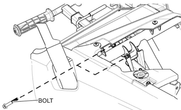
12. Place the radio mcu into the glovebox area. Line up the holes in the radio bracket with the holes in the grab handle bracket. Use the supplied 12 mm flange bolts to attach the radio mcu to the grab handle bracket. Tighten bolts to the specification supplied in the Torque Chart then reinstall the glovebox in the reverse order of removal.
