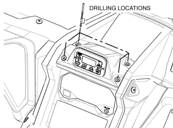
16. Place the radio controller cable drill template on the top of the instrument panel.
