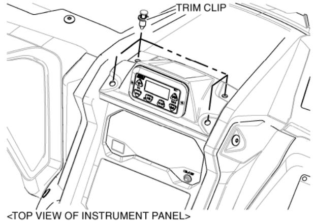
19. Using the trim clip removal tool, remove the five trim clips as shown below.
