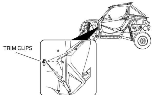
20. Using a trim clip removal tool remove 11 trim clips along the lower side cover. Remove the two hex head screws (as shown).
