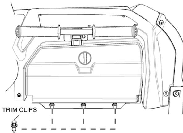
8. Slide the grab handle forward to full extension, open the glovebox and remove two 5 mm hex head screws and one trim clip then remove the glovebox. After the hardware has been removed, pull the glovebox out and away.
