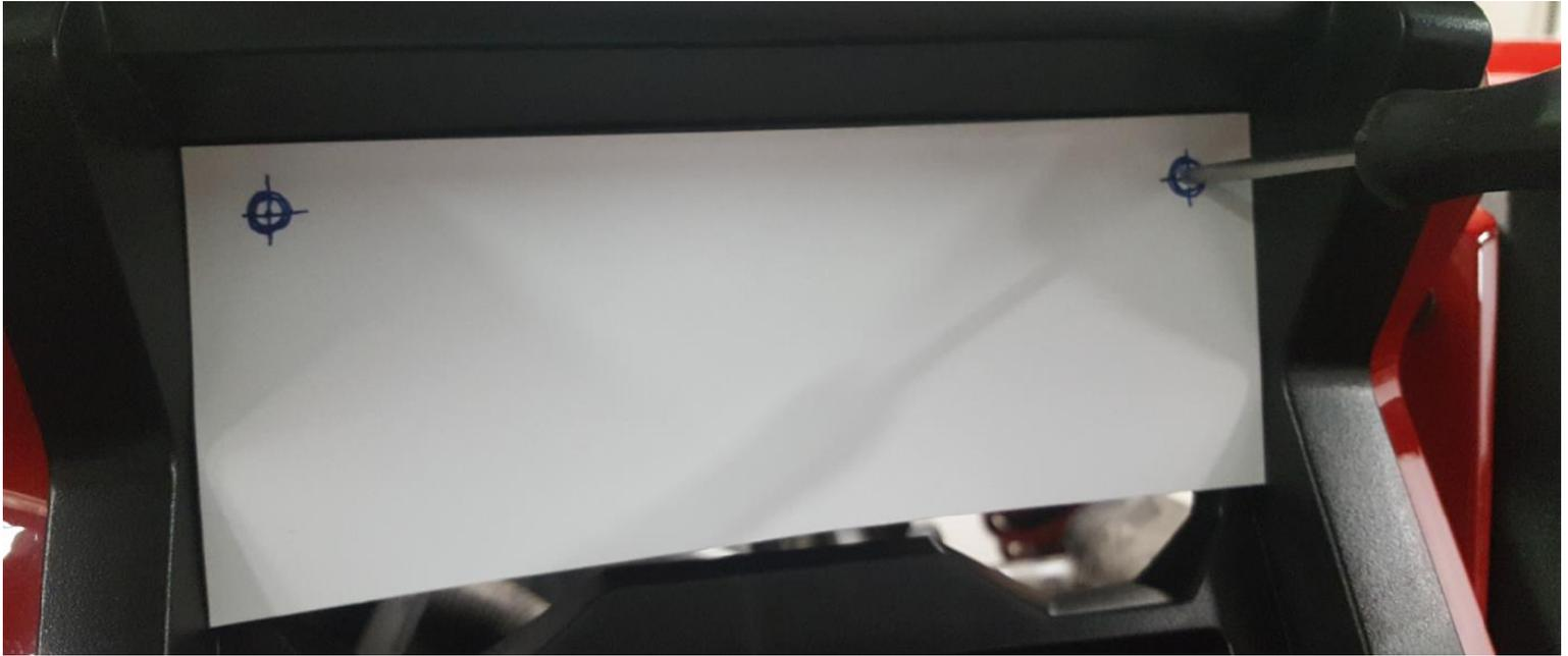
23) Fold the template and place it in the cubby hole. Use a sharp pick and punch a pilot hole into the top side of the cubby hole...
