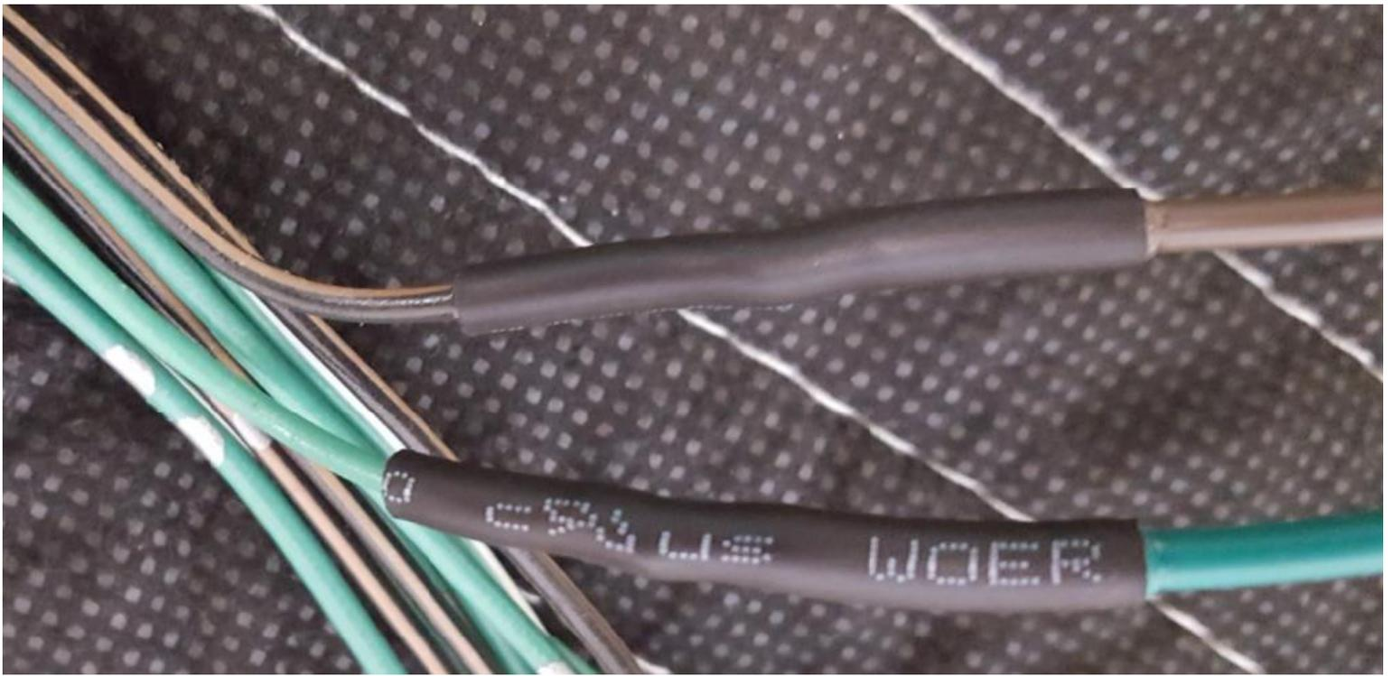
14) Route the wires through the harness, cut to length and repeat the splice on the other end. Rewrap the tape in the corners and in the middle to hold the harness together so you can rewrap it. (NOTE, if you have a Live Valve model, there will be another small harness. You will not need to do anything with this harness except reroute it from the driver side to the middle) ...
