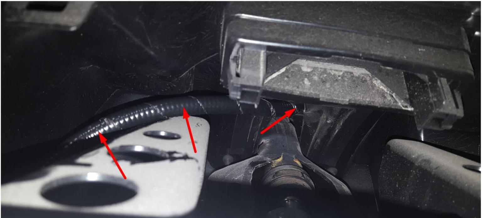
17) Remove the Allen head screw from the top of the steering column (do not remove the plastics)...
