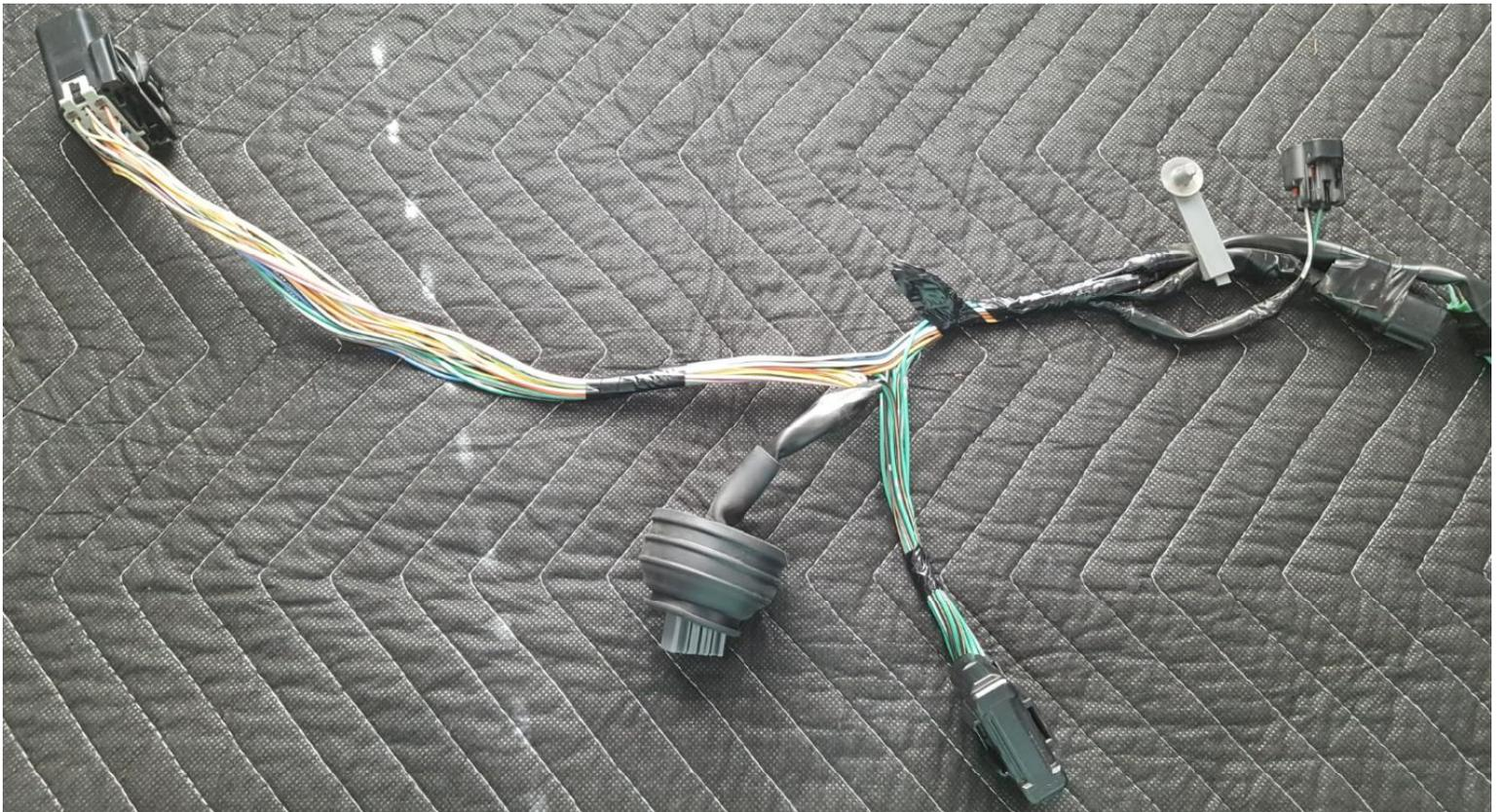
11) Pull the cluster plug away from the power/ground block and cut the 2 wires that are short. There will be one Black/Brown and one Green wire...
