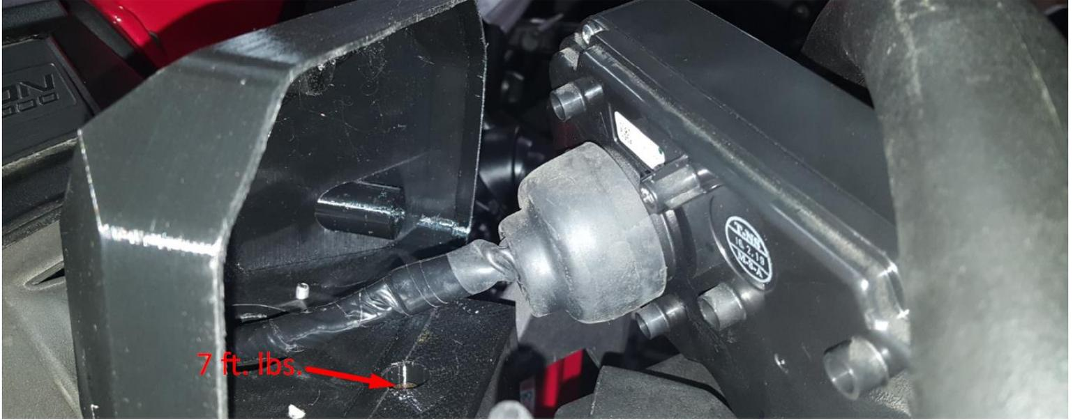
20) Install the Cluster and use a 1/4 drive Phillips bit, 1/4" socket and 1/4 drive ratchet to install the screws...
