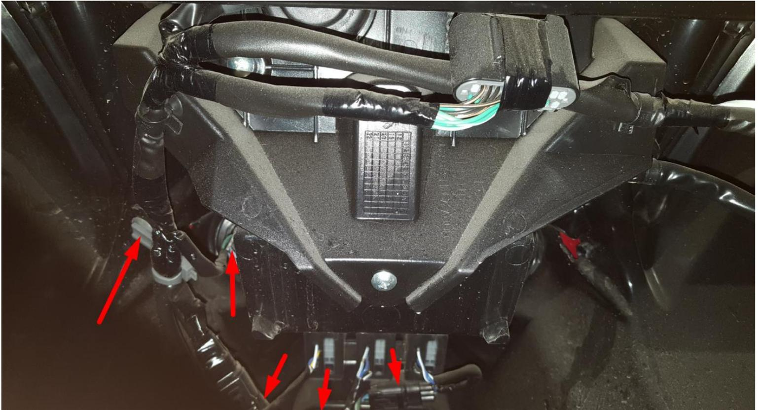
4a) IF you have a Live Valve model, there is one more wire loom clip to release and one more connector to remove just above the steering column...
