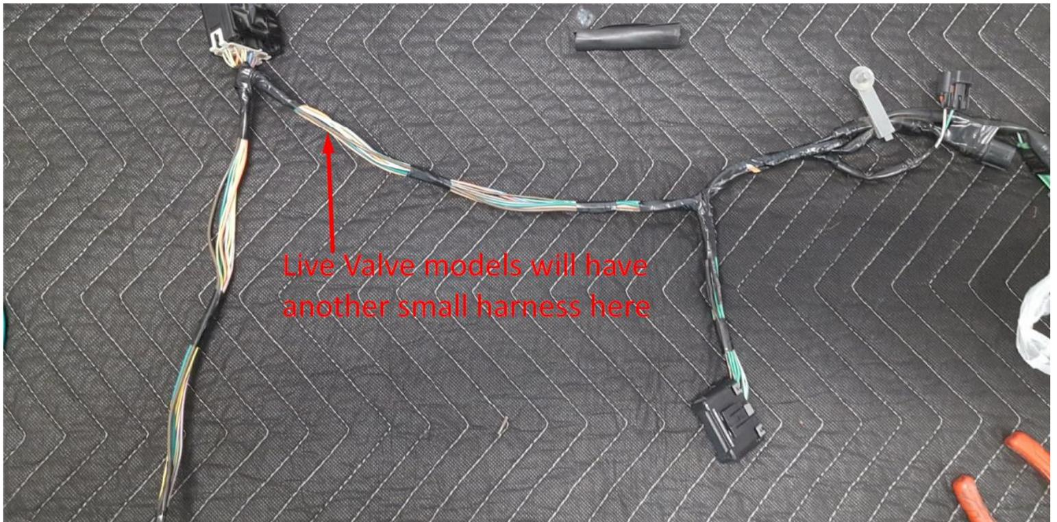
15) Reinstall the removed wrap and put supplied wire loom on the newly exposed part of the harness. Tape all the overlaps and tape the power/ground block to the harness. Your finished harness should now look like this...
