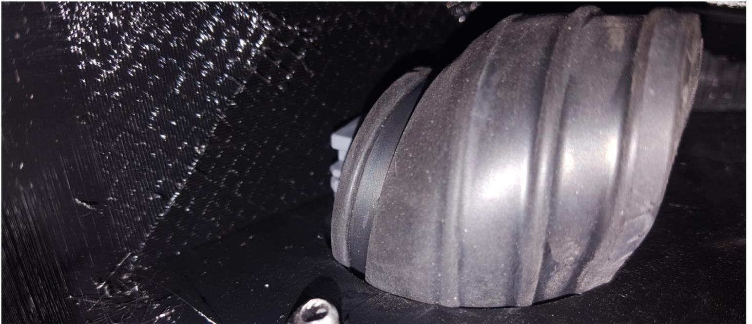
19) Place the cluster mount on the column and line up the hole. Place the supplied small head 6mm bolt in the hole, make sure to keep the cluster mount straight and tighten the bolt to 7 ft lbs (84 in lbs). Connect the Cluster and “roll” the boot back over the cluster...
