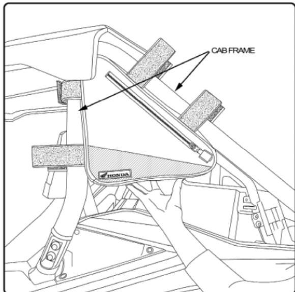
2. Loosely wrap one of the hook and loop straps around the upper cab frame. Start with the top straps then fasten the bottom straps.
