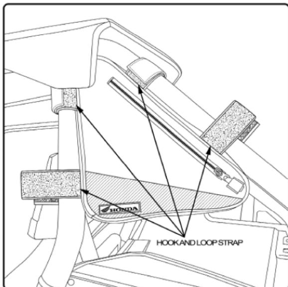
3. Tighten all the straps to secure the bag
