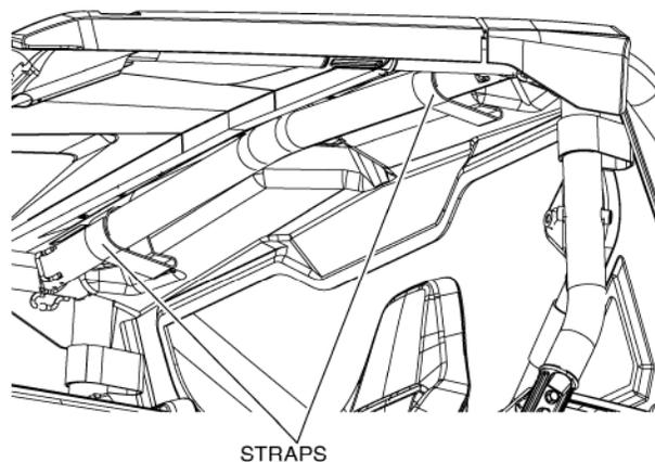
5. Wrap the remaining four straps around the top horizontal OPS bar.
