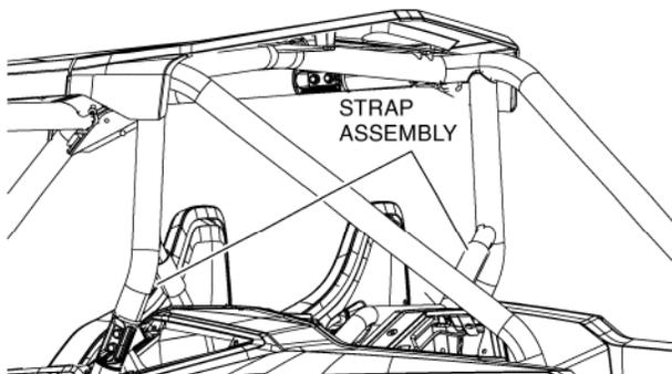
3. Place the Fabric Rear Panel behind the vertical OPS bars. Loosely wrap one strap around each vertical OPS bar.
