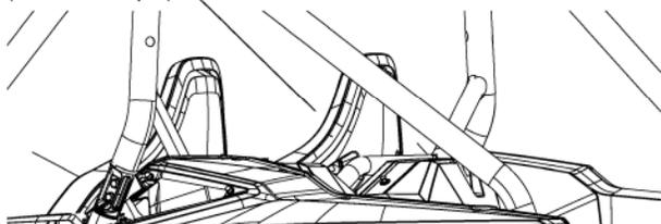
2. Install one Strap Assembly on the driver and passenger sides (as shown). Be sure the anti-slip side of the strap is facing inward.
