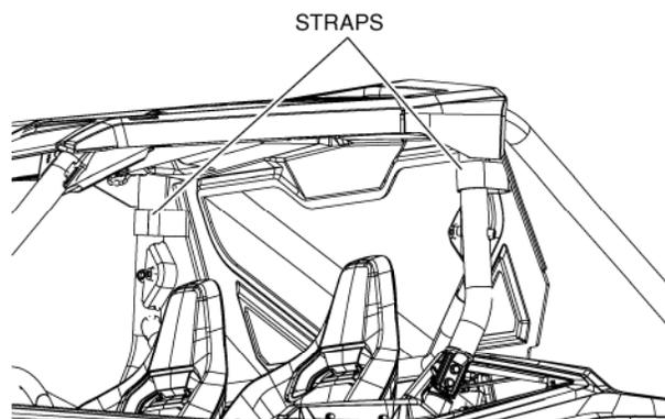
4. Wrap two straps around the top horizontal OPS bar to hold the Fabric Rear Panel in place (as shown).
