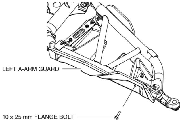
4. Loosely install the fender washers and the 10 x 25 mm flange bolts starting with the closest to the wheel.
