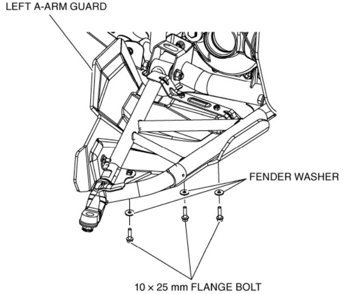
5. Tighten all the bolts the value specified in the TORQUE CHART starting with the one facing forward.
