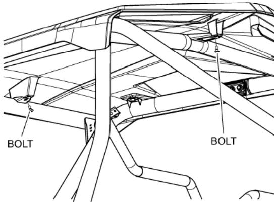
3. Loosely install the visor along the front edge of the OPS crossbar using two 20 mm hex head bolts, flat washers, and nuts. Do not fully tighten the hardware at this time.
