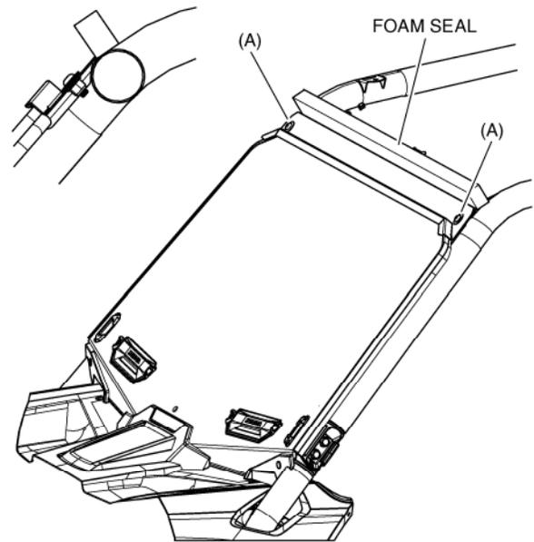
14. Attach the center bracket to the dash panel using two trim clips. Apply pressure to the outside of the windshield to allow the holes in the center bracket to line up with the holes in the dash panel.
