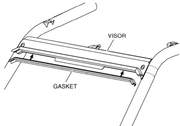
5. Locate the upper ends of the side gaskets on the windscreen. Lift the ends, then remove the paper backing from the adhesive strip. Firmly press the ends back down onto the edges of the windscreen as shown.
