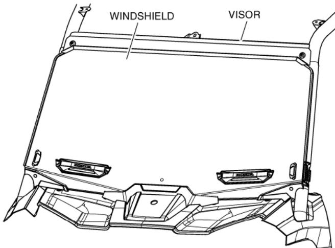
11. Make sure the knobs are fully inserted into the mounting clips, then turn the knobs 90 degrees clockwise to the position shown to secure the windscreen.
