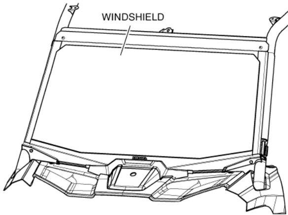
6. Line up the holes in the top corners of the windshield with the holes in the OPS. Reinstall the 20 mm hex bolts and Nylock nuts to attach the top of the windshield to the OPS as shown then tighten hardware securely.
