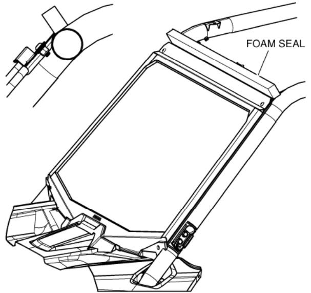
9. Loosely install the bottom of the windshield to the mounting clamps using one spacer, washer, and 20 mm hex bolt as shown. Repeat on the other side then tighten hardware securely.
