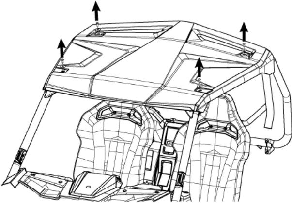
2. Remove the two bolts securing the roof from the inside of the vehicle. Remove the roof and set aside.
