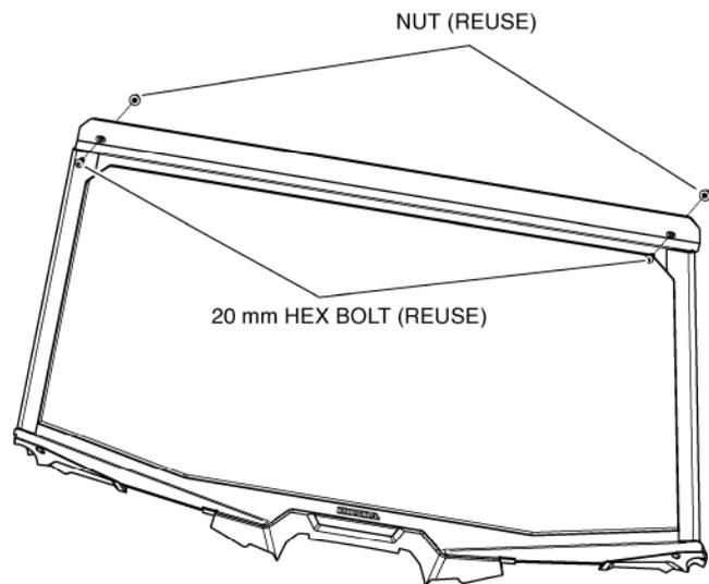
5. Place the windshield on the vehicle as shown. Press the windshield down to make sure the gasket is making contact with the top of the dash panel.
