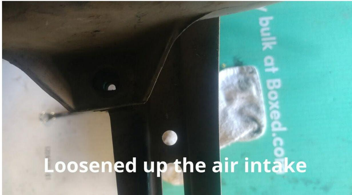
The manual has you removing snorkel duct A, which is the black plastic air intake tube that runs below your Pioneer. I didn't need to remove it to make room for the sub-trans to come out, but I did need to remove its fastener to the frame, just in front of the sub-trans. This allows you to shift it off to the side an inch or so. Until I did this, the sub-trans would bump into it and wouldn't slide off all the way:
