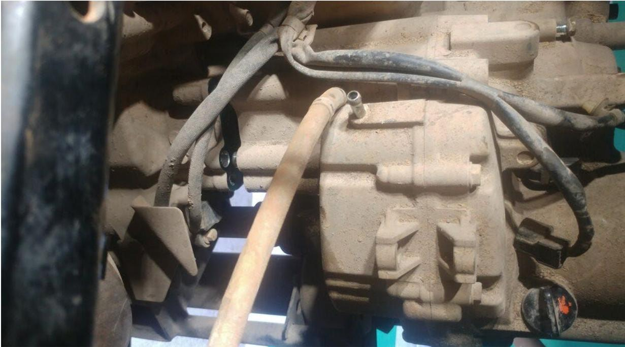
The manual (page 12-7, PDF 377) tells you to collect up your dowel pins, gasket, and drive damper. My drive damper blew up when the sub-trans came out, I don't know why. I had five springs falling out, snap rings, etc. I was able to re-assemble it on the bench, so it turned out OK.
