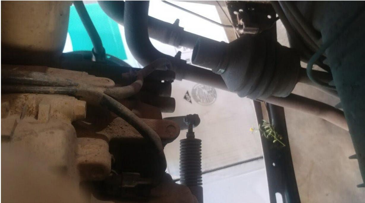
Move your driveshaft to the driver's side, on top of the cooling lines to get it out of the way.
