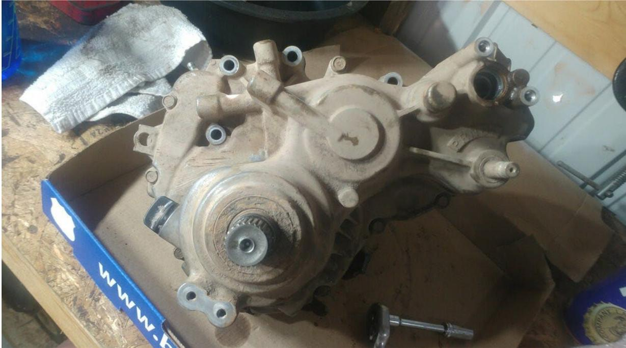
I tried to clean it up the best I could around the bolts and gasket before I opened it, using compressed air and a toothbrush. You'll be removing the ten bolts holding the cover on, and then tapping on it with a plastic or rubber hammer while separating it. I found I also needed to tap on the output shaft to get it to come free.
