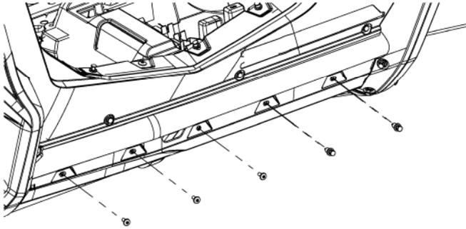
2. Install the sub frame as shown with the original hardware removed at step 1.
