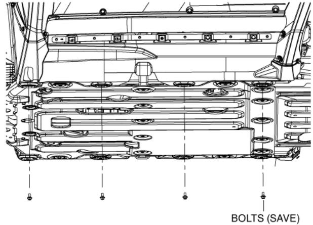
4. Loosely install the left side skid plate using the fender washers and the 10 x 25 mm flange bolts at the positions shown.
