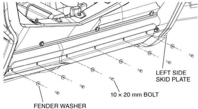
6. Tighten upper bolts first and then the lower bolts to the value specified in the TORQUE CHART.
