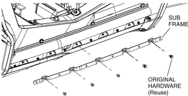
3. Remove the side panel lower bolts as shown.
