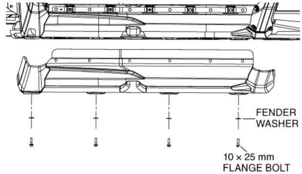
5. Loosely install the 10 x 20 mm bolts and fender washers to attach the left side skid plate on the sub frame as shown.
