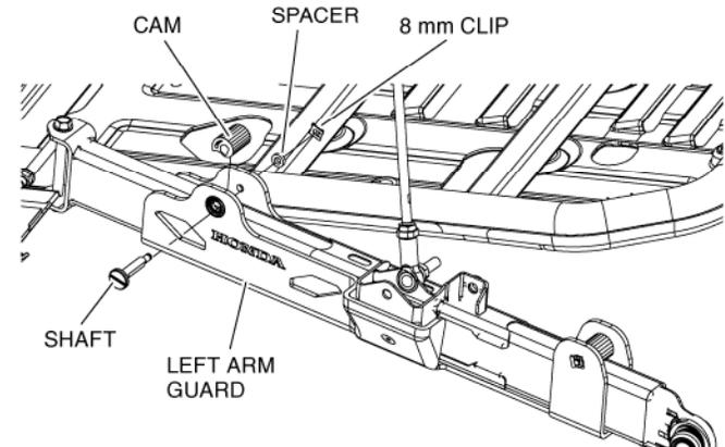
6. Tighten the shaft with the key.
