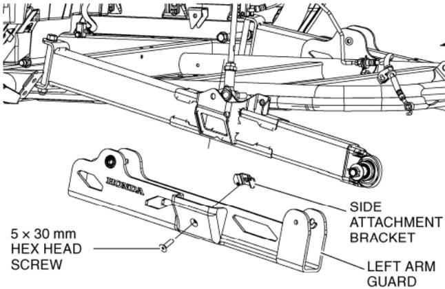
2. Position the side attachment bracket horizontally and insert the bracket through the rectangular hole in the rear arm of the vehicle.
