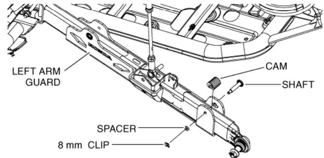
5. Insert the cam between the ends of the left arm guard and pass the shaft through with a spacer at the end. Use the trigger clamp to set the hardware assembly with the 8 mm clip as shown.
