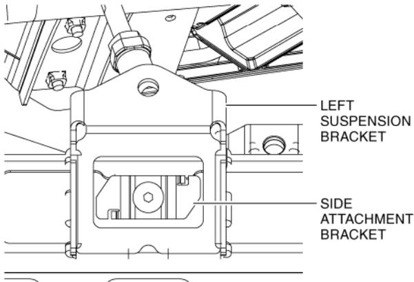
3. Rotate the side attachment bracket vertically and tighten the 5 × 30 mm hex head screw to the value specified on the TORQUE CHART.
