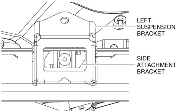
3. Rotate the side attachment bracket vertically and tighten the 5 × 30 mm hex head screw to the value specified in the TORQUE CHART.
