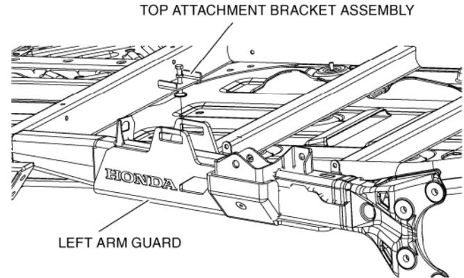
5. Place the top attachment bracket assembly on the left arm guard as shown below. Be sure to center the bracket assembly on the suspension arm then tighten the 10 mm bolt of the bracket assembly to the value specified in the TORQUE CHART.
