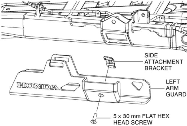
2. Position the side attachment bracket horizontally and insert the bracket through the rectangular hole in the rear arm of the vehicle.
