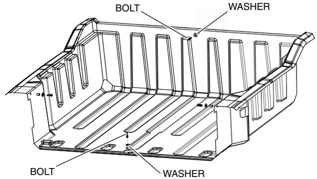
5. Install a collar, washer and bolt at the left and right locations.
