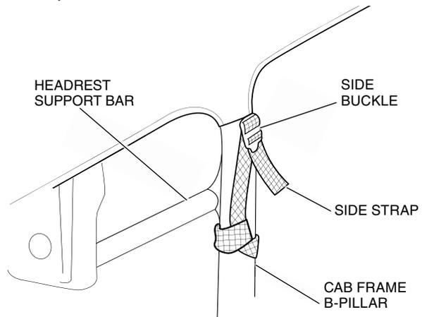
4. Wrap the rear side strap with side release buckle down behind the cab frame C-pillar, around the net bracket, and back up to the mating buckle as shown.
