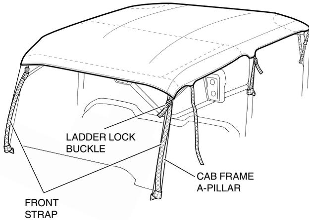
6. Wrap the rear center strap around the upper rear horizontal cab frame bar. Thread the strap through the buckle and back to itself as shown. Repeat for the other side. Tighten all the straps at this time (front, side, rear).
