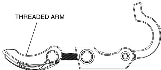
9. Swing the threaded arm over the top half of the clamp and snap the arm closed.
