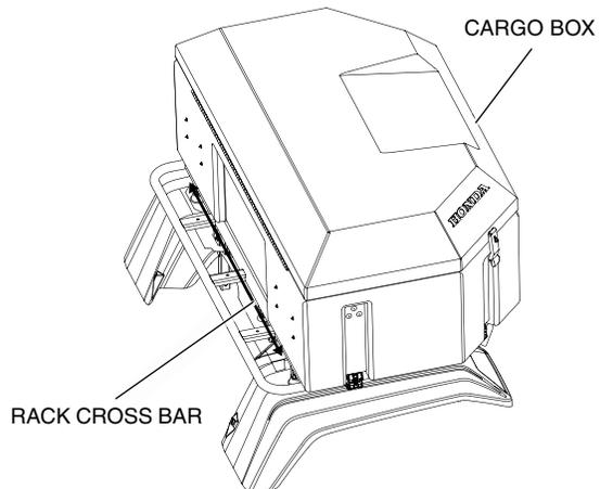
8. Align the clamps around the rack frame bars.
