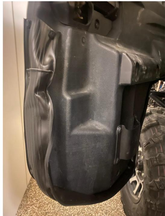
Step 3. The next step will repeat until you have the seal to the end of the door follow along the edges of the door and pull the seal till it is tight along the edge mark where the hole needs to be and drill out and attach the supplied push clip then move to the next hole on the seal. Pictures below should help in reference to the position it should sit on the door.
