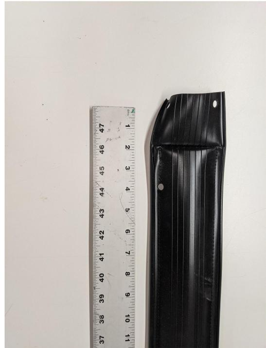
Step 2. Start the seal on the front of the door position it level to the bottom of the latch component (shown in picture to the right). Start drilling the holes just off of the center line as shown in picture below.
