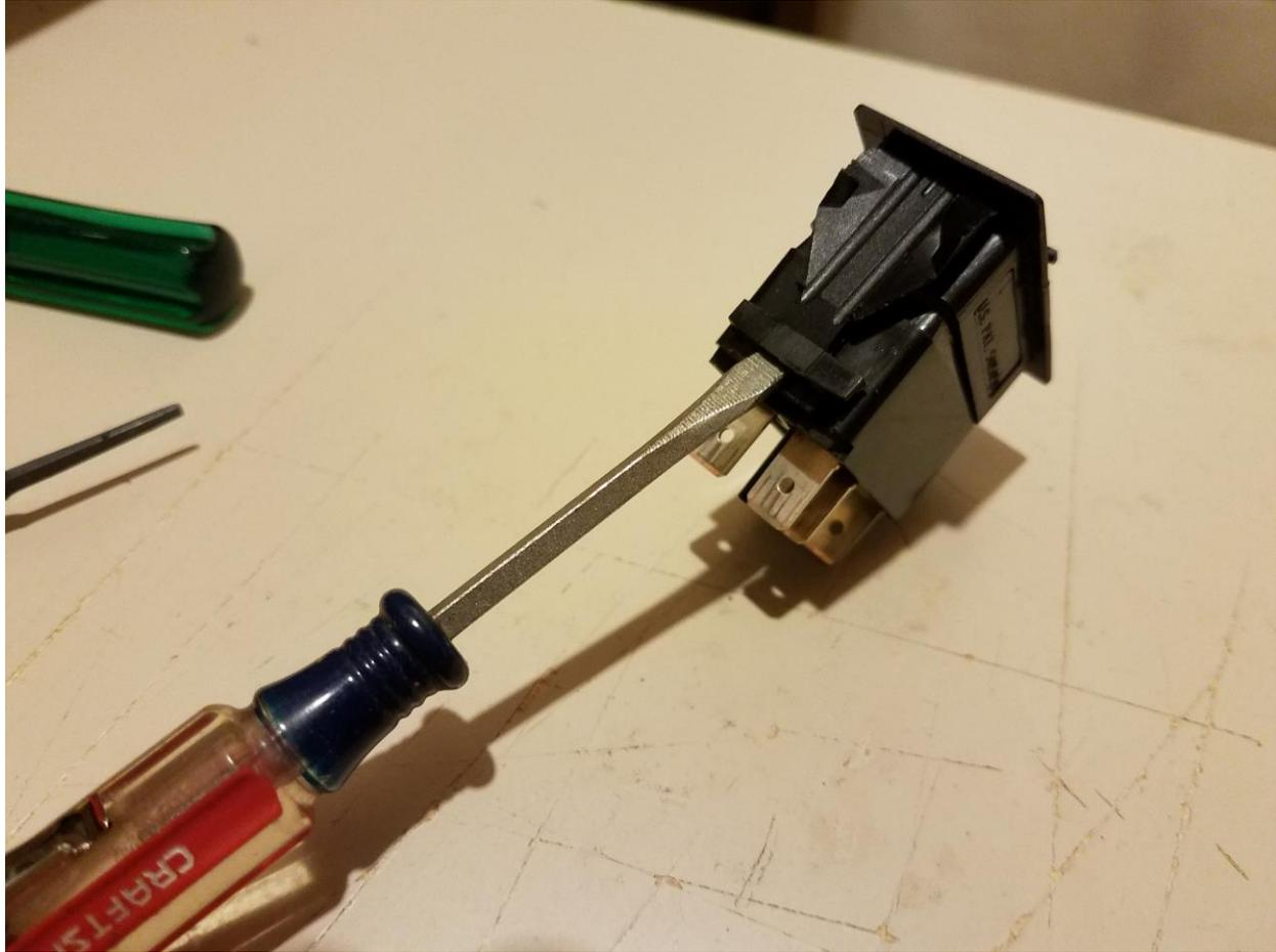
Carefully pry the tabs out, which will release the upper and lower bodies of the switch. Be careful, there are 4 springs which will pop the switch open once the tabs are released. There are several parts that will easily fall-out once the 2 halves are separated. It is not difficult to put back together, just don't lose any of the pieces.
