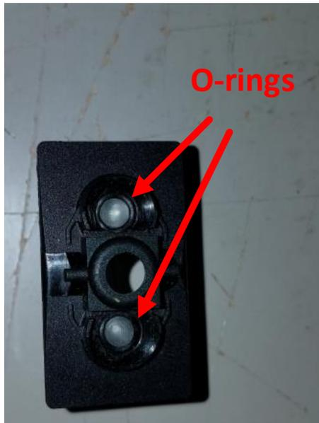
With this style of Rocker switch, some of the light bleeds around the rocker. This is not a big deal, but it is more noticeable when it is dark in the cab. I found a post by Hondasxs where he added a foam gasket between the Rocker and Switch body. This
