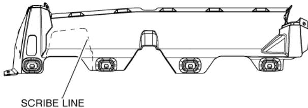
5. Reinstall driver and passenger side skid plates onto the vehicle. Use care to ensure the hooks on the rear over fender are installed into the slots on the driver and passenger side skid plates.
