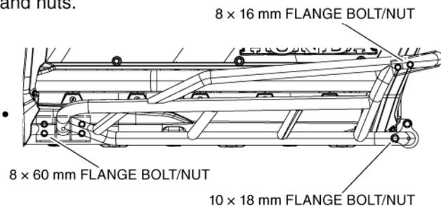
7. Tighten the 8 mm bolts in Area 1, then Area 2, then lastly tighten the 10 mm bolts in Area 3 (as shown). Tighten bolts/nuts to values shown on the Torque Chart.
