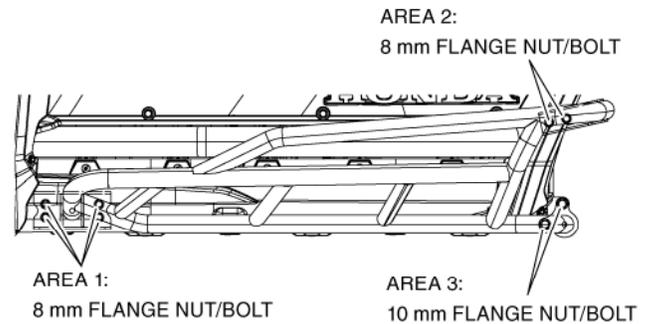
8. Install the passenger side nerf bar by repeating steps 6 and 7.
