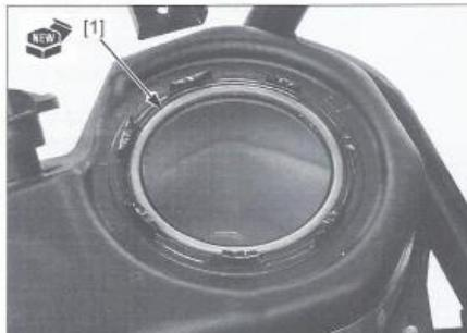
*Be careful not to damage or pinch the O-ring.*
