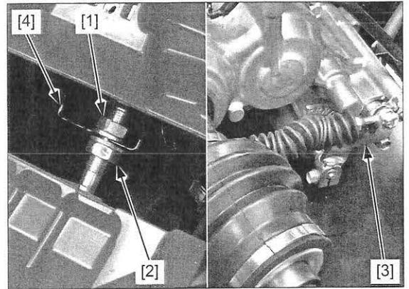
Adjust the shift select lever freeplay when the indicator indicates "N" (neutral) by turning the adjusting nuts [1].
