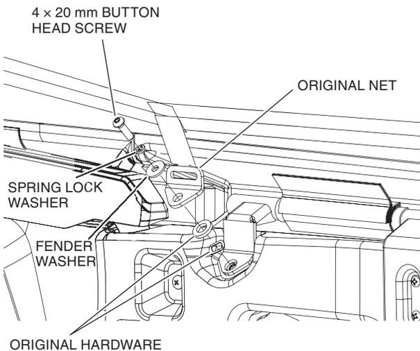
14. Install the original net on the door using the original hardware (as shown).
