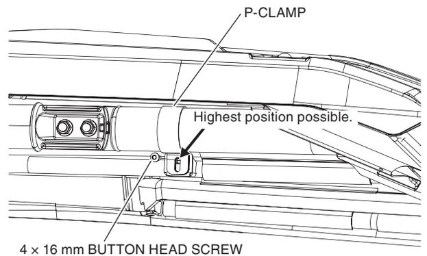
11. Wrap the upper strap on the Fabric Upper Door around the vertical OPS at the highest position possible then tighten.
