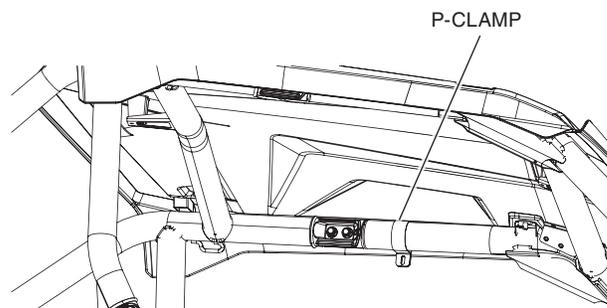
5. Install two C-clamps on the vertical OPS tube (as shown).
