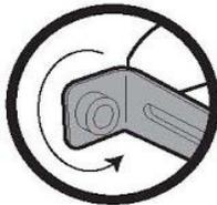
When installing, rotate L-Brackets so that the arm is facing inwards, towards the intercom/radio slots
